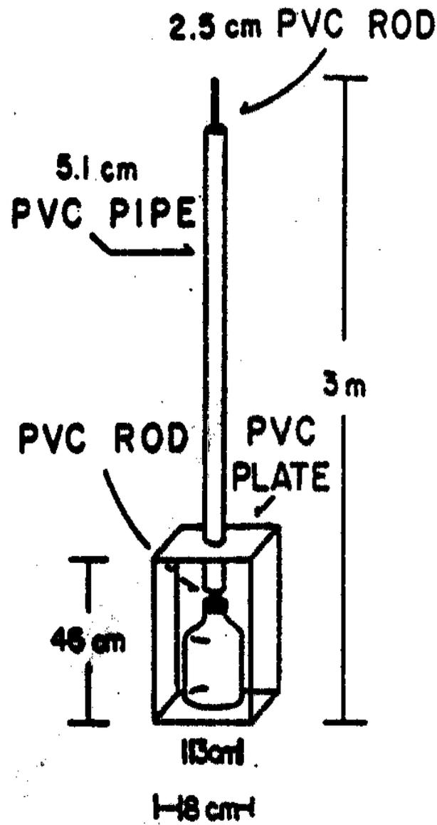
**Figure 3 - Jar Sampling Device**
